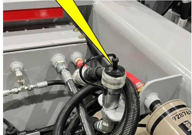
Hydraulic Fluid Drain Port
